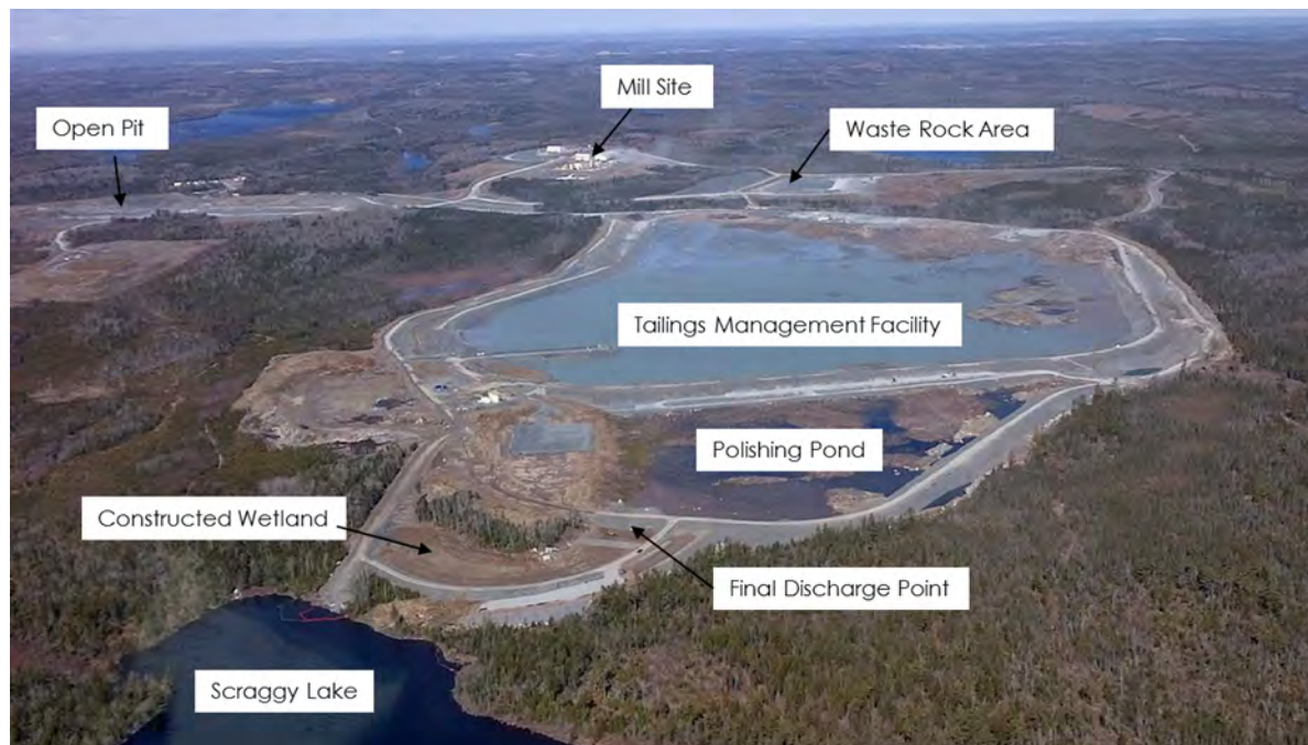
Photo 1 Touquoy Gold Mine in Moose River Gold Mines, NS. View is looking to the north-northwest.
